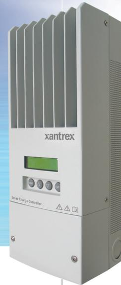
The Xantrex™ XW Solar Charge Controller is a photovoltaic (PV) charge controller that tracks the electrical maximum power point of a PV array to deliver the maximum available current for charging batteries. When charging, the XW Solar Charge Controller regulates battery voltage and output current based on the amount of energy available from the PV array and state-of-charge of the battery.
